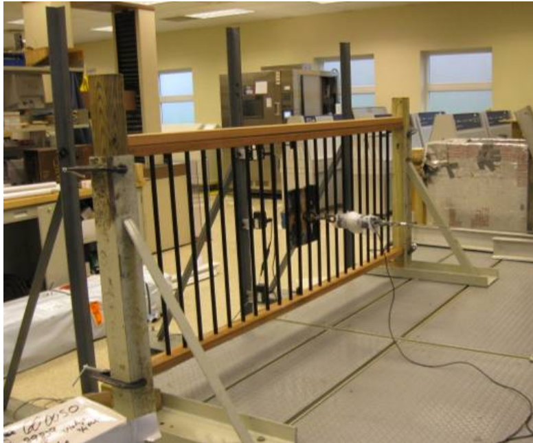
Photo No. 7 In-Fill Load Test at Center of Three Vintage Series Round Style Balusters (Installed with EZ Mounts)
