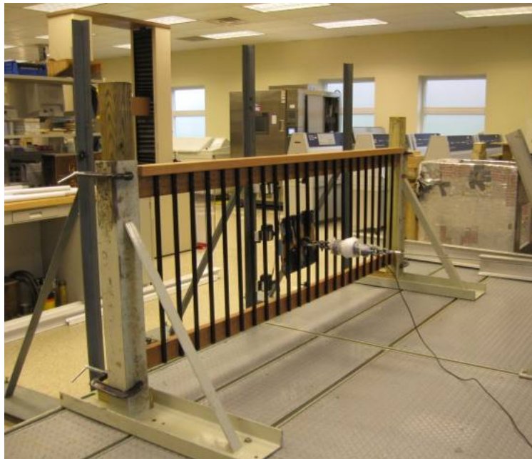
Photo No. 4 In-Fill Load Test at Center of Three Vintage Series Square Style Balusters
